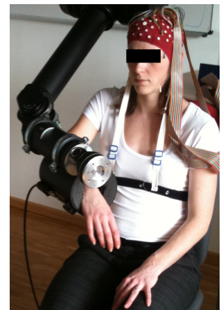
Fig. 1. A robot arm is attached to the patient's forearm and it may move the patient's forearm with the elbow as the single degree of freedom (DoF). The resting position, maximum extension and maximum flexion of the robot arm can be adjusted depending on the patient (adapted from [20]).
